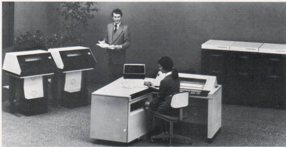
The B80 with three disc units, two printers and four cassette drives.
